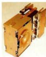
4.5 kV, 3.5 kA Switch Plate
