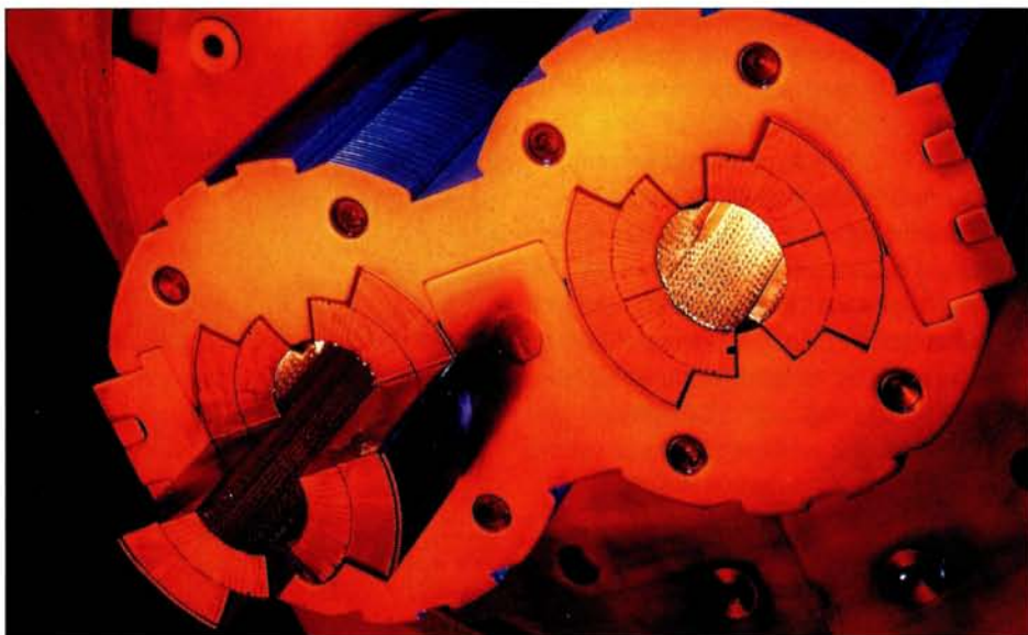
This early engineering model of an LHC dipole shows the concept of the austenitic steel collars that surround the superconducting coils.
